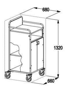
Multipurpose trolley divided into two parts, one for clean laundry and one for dirty laundry, separated by a vertical wall.
