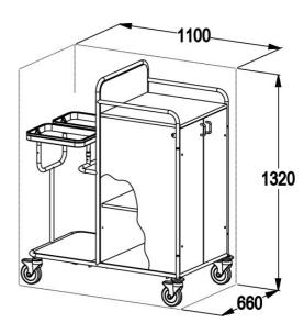
Multipurpose trolley divided into two parts, one for clean laundry and one for dirty laundry, separated by a vertical wall.
