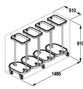
Rigid, sturdy, self-supporting ABS plastic base with edges to contain any leakage from the bag. The bag holding ring(350x255 mm) is made of glass reinforced nylon with a rubber gasket hot-injected onto it to ensure it is an integral unit with no gaps, making it easier to clean and ensuring cleanliness and hygiene. The gasket holds the bag in place so it can not slip out
